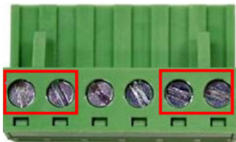
Figure 2.5 - Power Terminal Block
