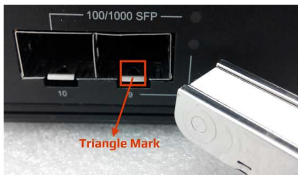
Figure 2.7 - Transceiver to the SFP Slot
