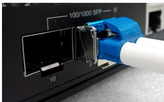
Figure 2.9 - LC Connector to the Transceiver
