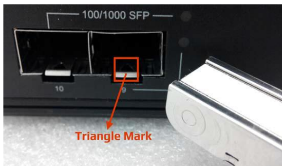
Figure 2.7 - Transceiver to the SFP Slot
