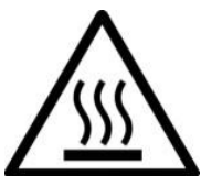
Figure 1.2 - Hot Surface Warning Label
