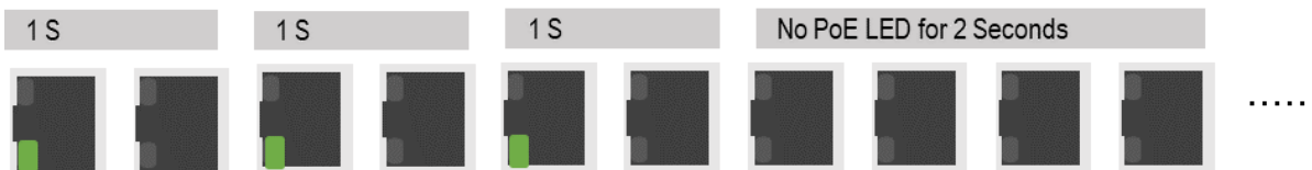
Figure 2.8 - PoE Cable Short Recovering LED Sequence
