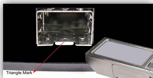
Figure 2.7 - Transceiver to the SFP Module
