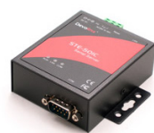
STE-501C 1-Port RS-232/422/485 To Ethernet Device Server
