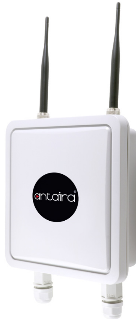
ARY-7235-AC-PD Industrial Outdoor IP67 Plastic Housing IEEE 802.11a/b/g/n/ac Wireless Access Point/Client/Bridge/Repeater/Router with PoE PD
