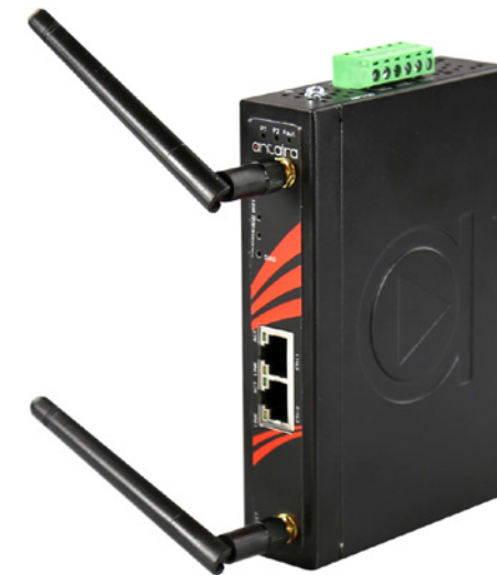
ARS-7131(-T) Industrial 802.11a/b/g/n WiFi Access Point/Client/Bridge/ Repeater/Router
